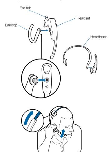
6 The ear tab has been designed to maximize stability of the headset. It can be rotated on the headset to optimize its fit and comfort in the ear. If desired, the ear tab can be removed by pulling tab from the headset.
